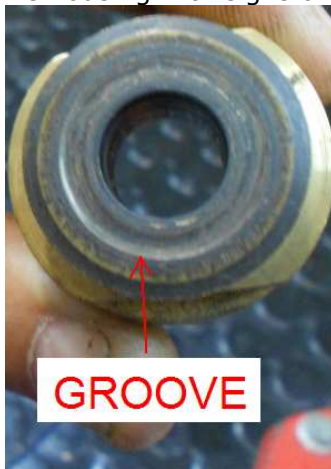
Valve housing with signs of wear
