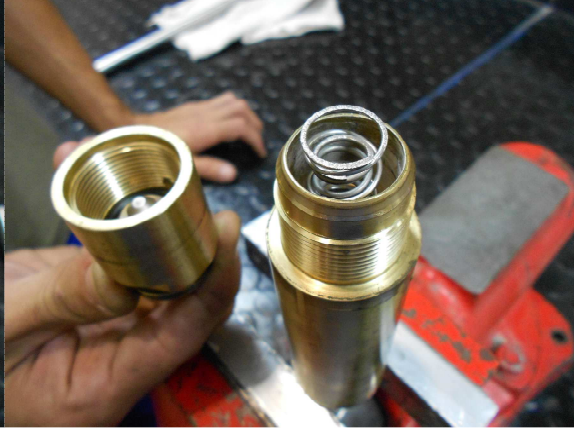
Removed seal tensioner and springs with no sign of damage
