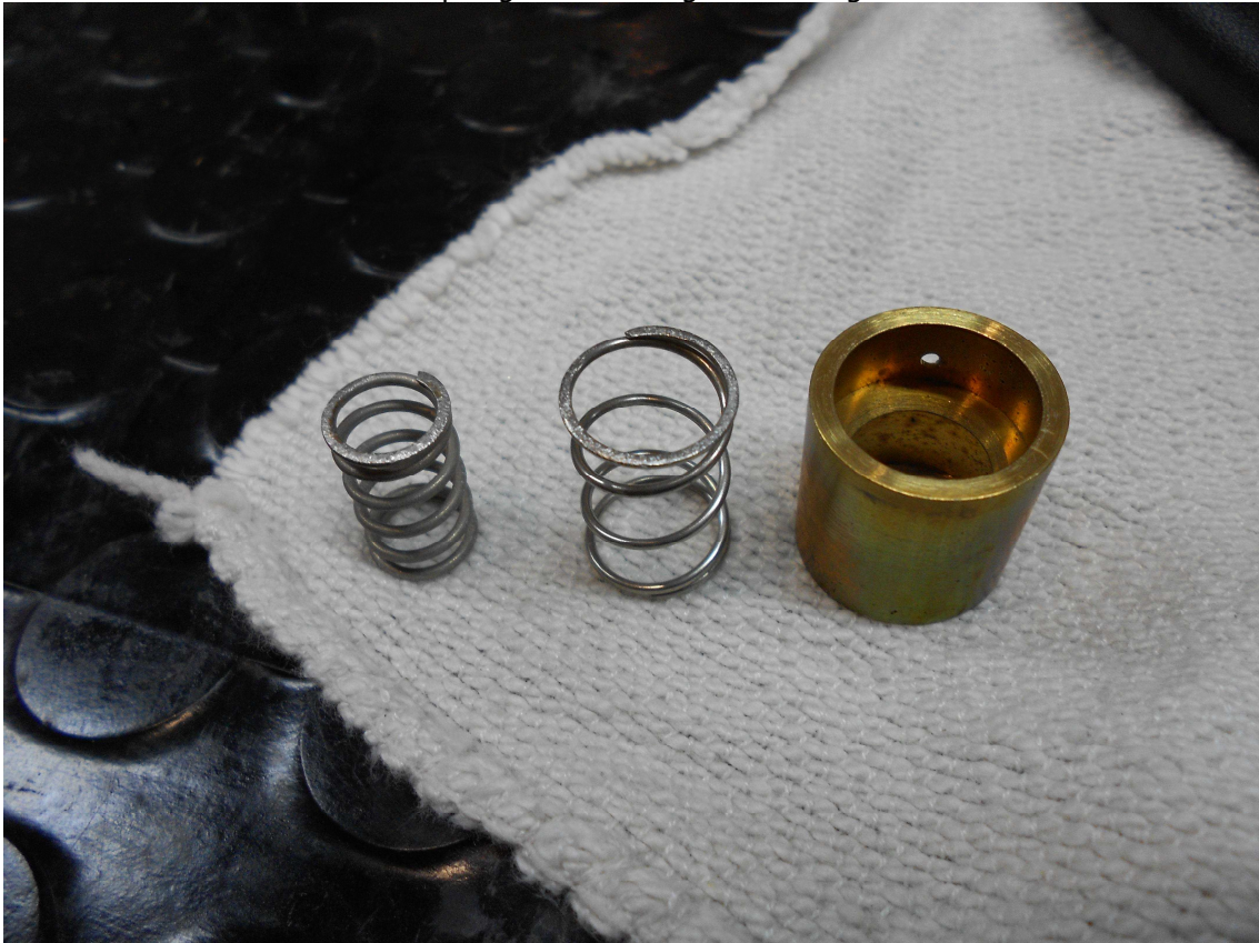
Removed seal tensioner and springs with no sign of damage
