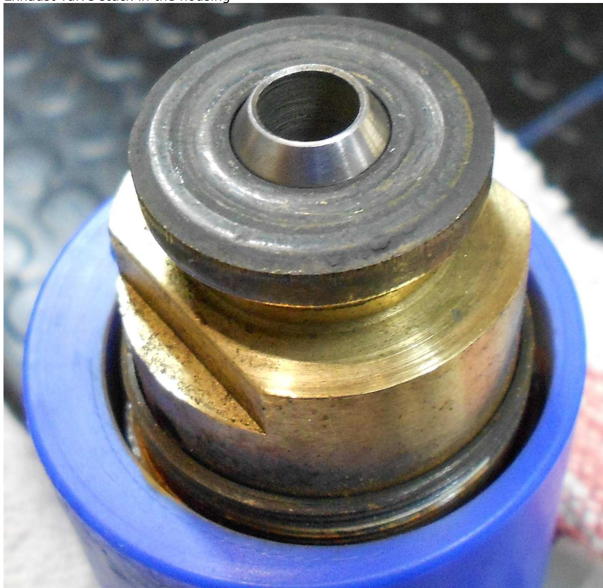
Exhaust valve stuck in the housing
